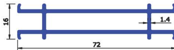
SECTION No : 6317 WEIGHT Kg/Mtr 0.674
